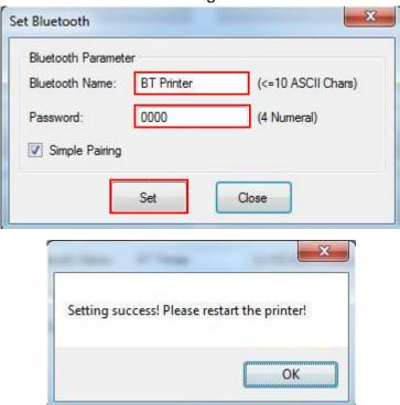
Note: When the "simple pairing" is checked, the printer does not need to enter the Bluetooth password to connect, when the "simple pairing" is not checked, the printer needs to enter a Bluetooth password to connect.
