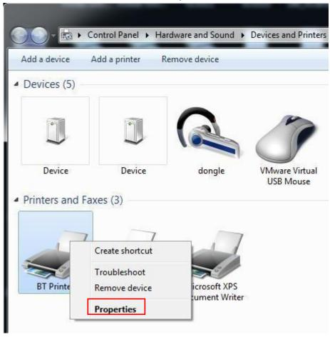
7. In the BT Printer properties, choose "Services", you can find COM3, that is connected to the Bluetooth port.
