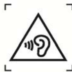
Figure 1 – Warning label (IEC 60417-6044)
