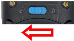
2. Grab the battery cover from the two recesses and gently lift upward, stop when you feel a resistive force. Press the battery cover against the battery, and lift the battery upwards until you remove the battery.
