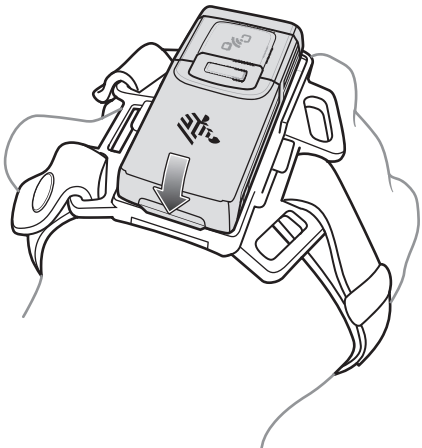
Figure 57 Push Down To Snap In Place
